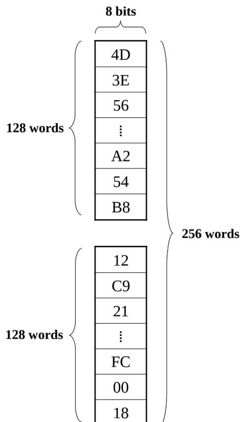
We can see these two memories (with a depth of 128 each) as only one memory (with a depth of 256).
