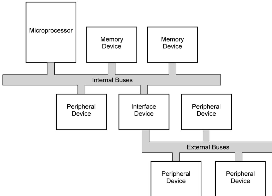
A bus is a collection of wires used to transfer information between components inside a computer. For instance, an 8-bit bus is made up of 8 wires and can transfer 8-bit values.
