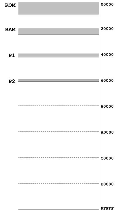
For instance, when the microprocessor sends the value  $403A6_{16}$  to its address bus, the address  $3A6_{16}$  of **P1** is selected.
