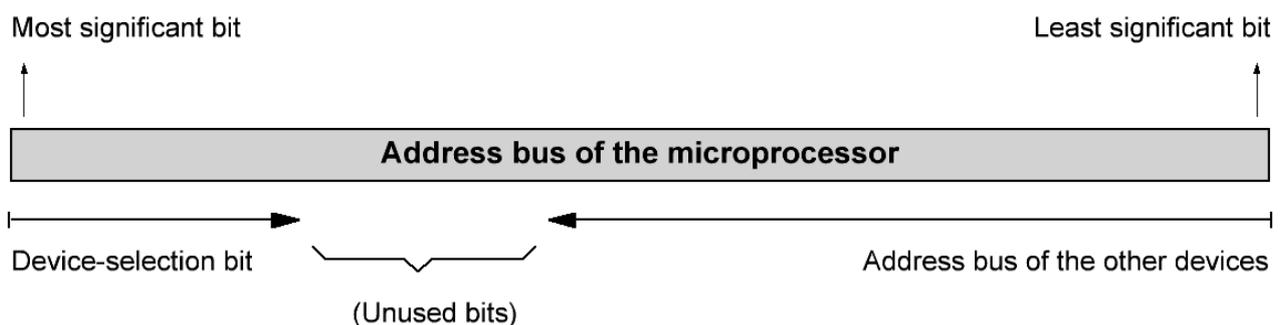
In some configurations (number of devices, size of the address bus, etc.), some bits of the address bus may be unused. For the time being, these bits will be set to zero.
